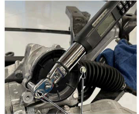
TORQUE BOLTS 8 N·m (6 lb-ft)
