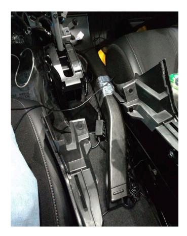
(The picture below) This portion is not recommended to cut because the airflow will weaken in the Rear AC Vent. It is better to leave it untouched so no air will flow in the foot vent under the front seats which is useless since we have now the air coming from the middle.
