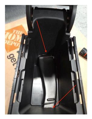
Use a plastic cutting tool or Dremel tool to cut a slot. You may polish the rough edge
