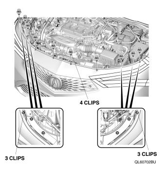
5. Remove the self-tapping screws, clips, and bolts.
