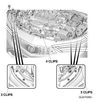
4. Remove the self-tapping screws, clips, and bolts.
