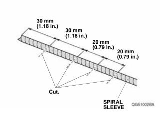
10. Place the spiral sleeves around the roof basket center bars as shown.
