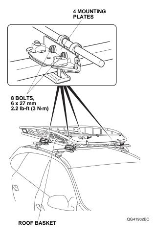
13. Attach the bracket covers to the mounting plates with lock plugs as shown.
