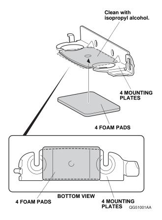
6. Attach the foam pads to the bottom of the mounting plates as shown.
