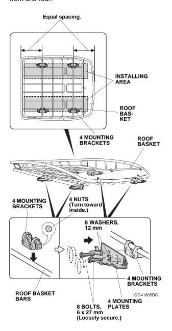
8. Loosely secure the mounting plates to the mounting brackets with the 6 x 27 mm bolts and the 12 mm washers as shown.
