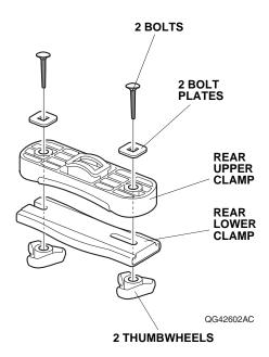
2. Remove the end cap, and slide the rear clamp assembly into the bicycle attachment as shown. Then, install the end cap.
