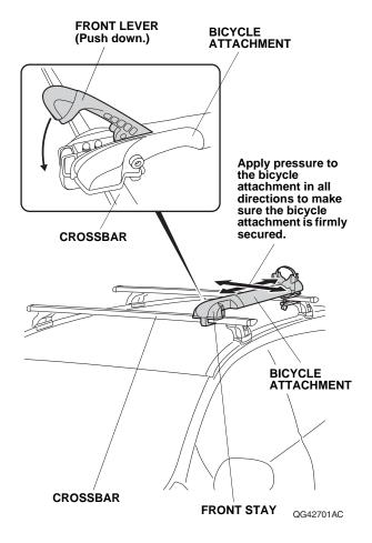
11. Grab the bicycle attachment, and try to move it side to side and front to back. If it moves, tighten the front stay and rear clamp until the bicycle attachment does not move. 12. Push the fork skewer through the front stay.
