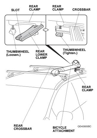
6. Place the bicycle attachment on the crossbars. Swing the rear lower clamp under the rear crossbar, and secure it as shown. Use the torque tool to finish tightening the thumbwheel.
