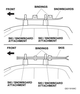
16. There are three different clamp catches, push down firmly on the ski / snowboard attachment top clamp to make sure that you get the proper clamp force.
