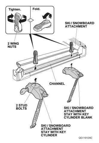
7. Tighten the wing nuts down on the ski / snowboard attachment stay stud bolts. Fold the wing nut handles flat down into the channel on the ski / snowboard attachment clamp base.
