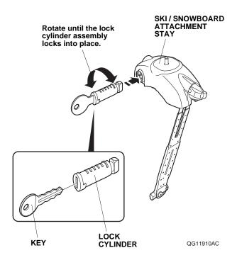
5. Place the lock cylinder blank into the ski / snowboard attachment stay.
