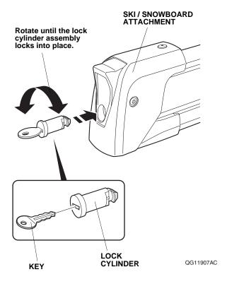
2. Unlock the ski / snowboard attachment and depress the latch to open the ski / snowboard attachment top clamp.
